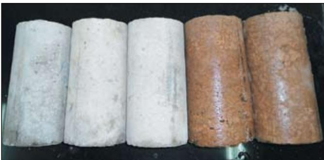
Figure 2. Concrete cylinders using OPC, LC3 A, B, C and D (from left to right) cast in the lab
