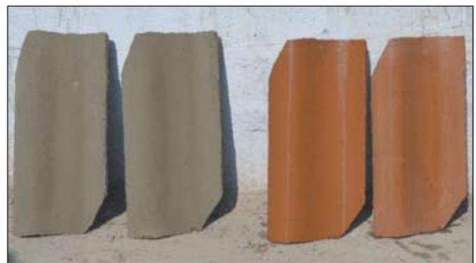
Figure 4. MCR tiles produced using LC3 A, B, C and D (left to right)
